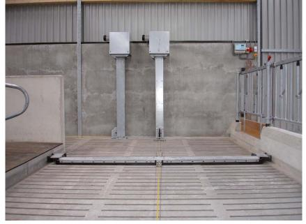
• This picture shows the complete system with 2 drive units mounted on consoles and the control panel above the feed front
